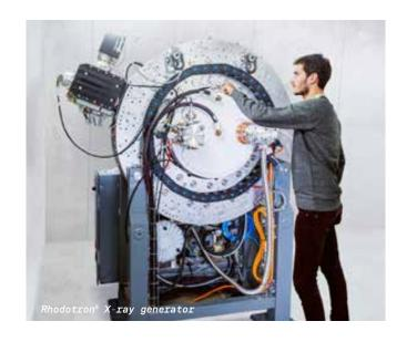
The IBA Industrial X-ray generator, based on Rhodotron® technology, is the key component of a new type of container control system installed in the port of Boston, in the United States. This advanced, non-intrusive system for inspecting cargoes is designed to detect, localize and identify contraband and security threats.
